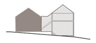
Using a slope to reduce height of two storey rear additions
